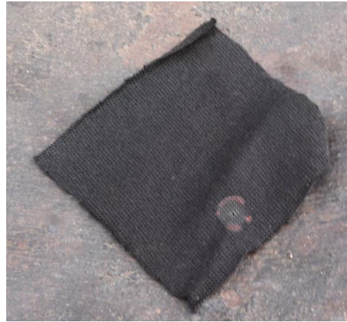
Charcloth hit with one spark from a steel striker against a flint
