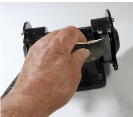
Flint against a grinding stone No sparks occur
