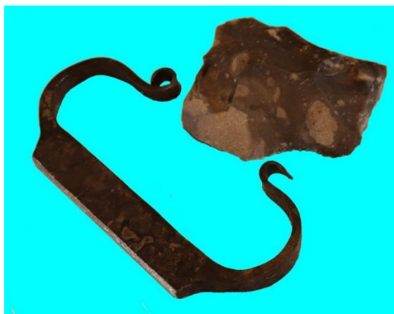
A piece of steel struck with a sharp flint will produce a spark
