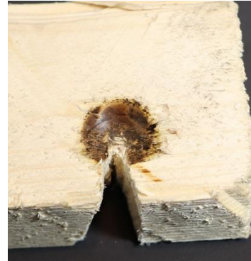
Step 3: Using a saw, cut a notch leading up to the hole
