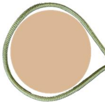
Smooth round spindle with slippery cord can slip
