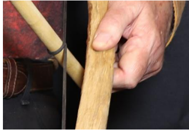
Twist the spindle to wind one turn of the string around the spindle
