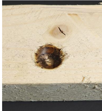
Step 2: Using your bow and spindle burn the indentation to get the hole more defined.
